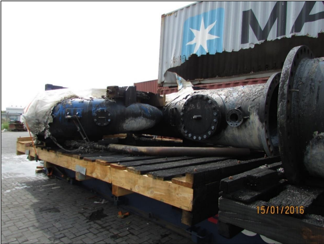
Tembat Spiral cases after unexplained fire on board during shipment from India to Malaysia.
